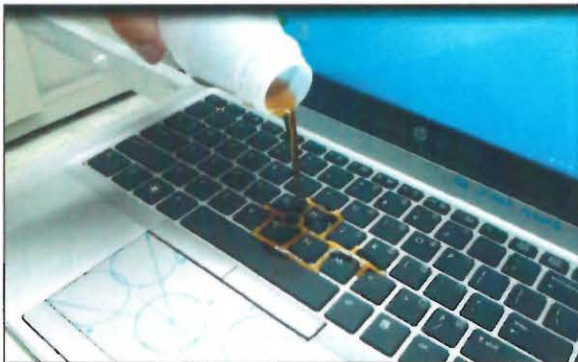
Coffee spill / drain test
